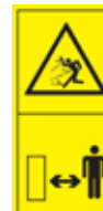
6 - Part # A77 DANGER Risk of injury to the legs. Keep a safe distance from the machine.
