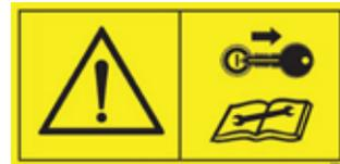
F -- Shut off engine and remove key
