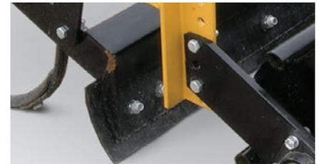
The double beveled leveling bar cuts the peaks and fills the valleys across the arena surface without packing it. The adjustable height allows operators to make fine adjustment to the material thickness increasing or decreasing cushioning.
