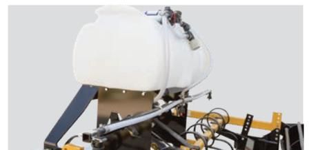
Equipped with a 25 gallon tank, the optional sprinkler kit reduces the amount of dust being thrown into the air when working with dry material.
