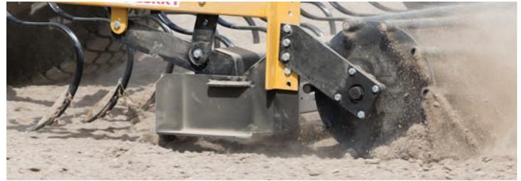
Every MK Martin Track Curry comes with two standard spill plates. These funnel any excess material into the Track Curry's path, ensuring your arena or track keeps looking its best.
