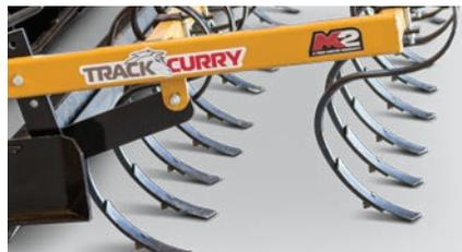
The two rows of S-tines works to loosen the material in your riding arena bringing the lower layer material to the top as they pull through ground. The S-tines are equipped with replaceable tips for easy maintenance and optimum performance.
