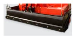
A 3PH pull type Meteor snow blower can be equipped with an optional hydraulic scraper. Equipped with corner markers so you always know it's position, the scraper allow you to pull snow away from doorways and structures so you don't miss a thing.
